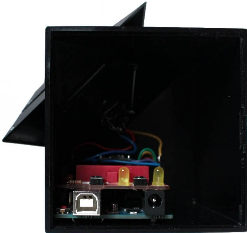
Figure 37 TimeCube with the Arduino board
