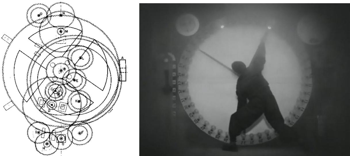
Figure 4. (left) complete mechanical schematic of the Antikythera device obtained by 3-d imaging (right) scene of the Metropolis film (1927)
