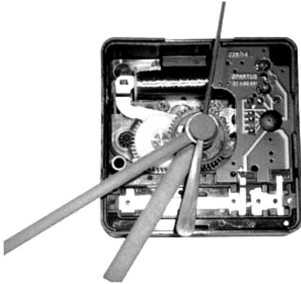
Figure 36 Photo of a quartz mechanism
